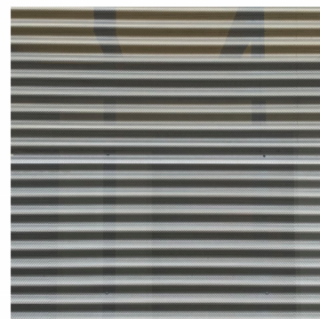
3. PERFORATED CORRUGATED SILVER METAL STAGGERED ROUND 1/8" DIA 3/16" CENTERS 40 % OPEN AREA
